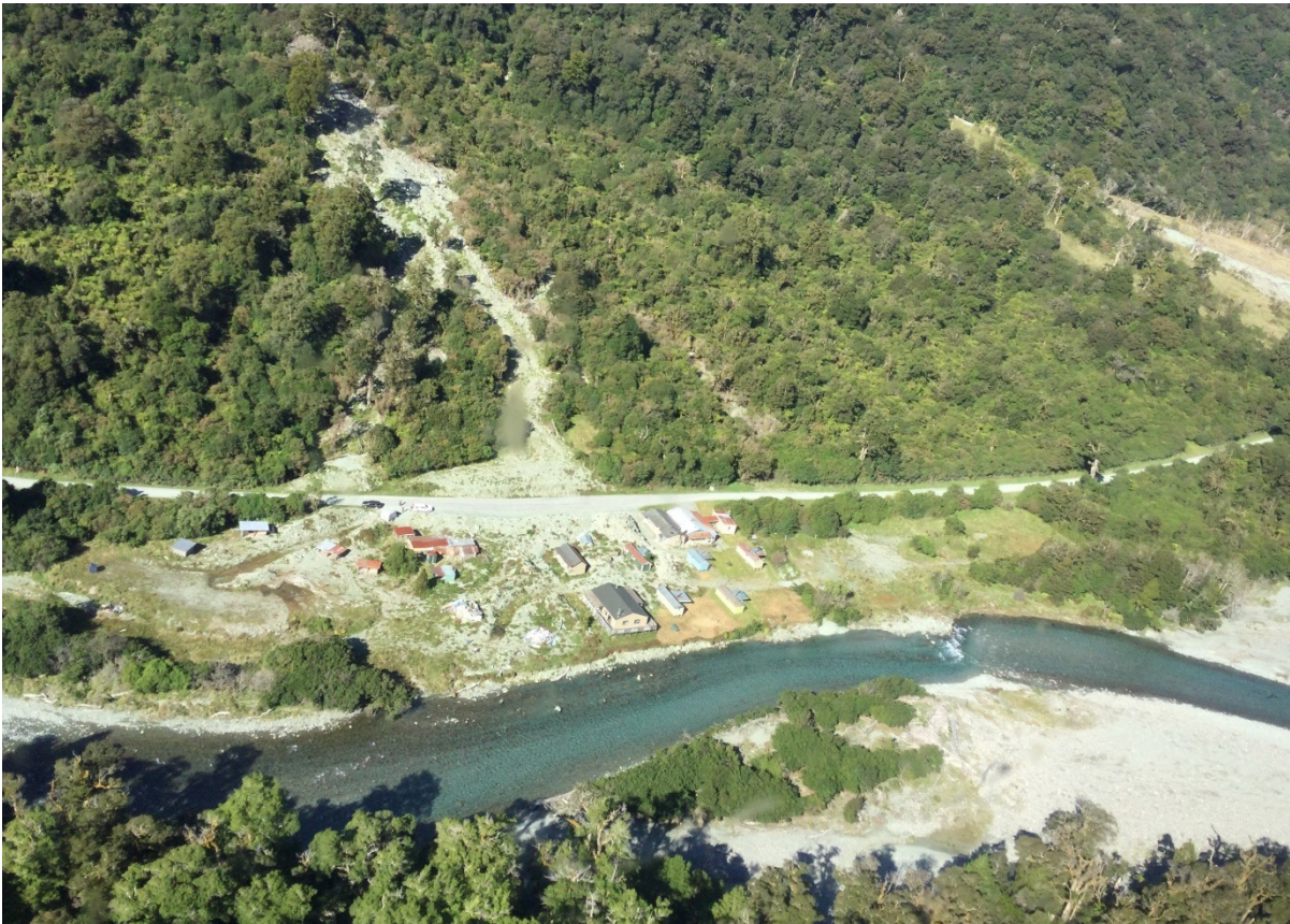
FIGURE 38: Changes in vegetation type at Gunns Camp, Fiordland. The lighter vegetation, generally to the right of the active channel appears to be of similar size, and likely points to regrowth following a very large debris flow event. Darker, and taller vegetation to the left of the active channel is at least partly old-growth forest, suggesting hundreds of years since inundation in this area.
