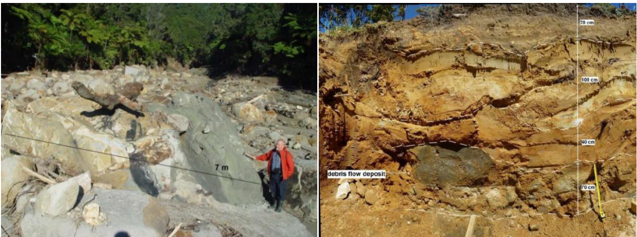
FIGURE 21: Left - Very large boulder (megaclast) within mix of sand, gravel, cobbles and boulders material deposited from the 2007 Matata debris flow (McSaveney et al, 2005); Right - Debris Flow Deposit overlain by Clay and Silt / Sand horizons (Page et. al, 2012).
