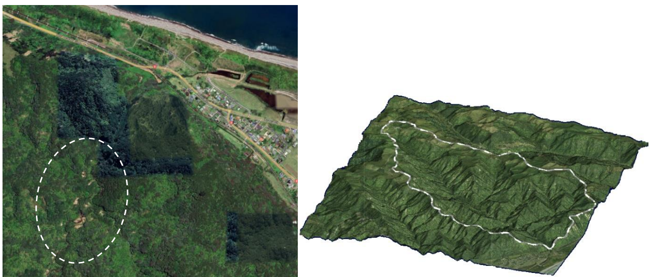
FIGURE 29: Matata Catchment Activity – Aerial imagery review: The large majority of the catchment is well vegetated (right), but there is evidence for a number of active or recent landslides within the catchment (left), possibly suggesting a Moderate Catchment Activity.
