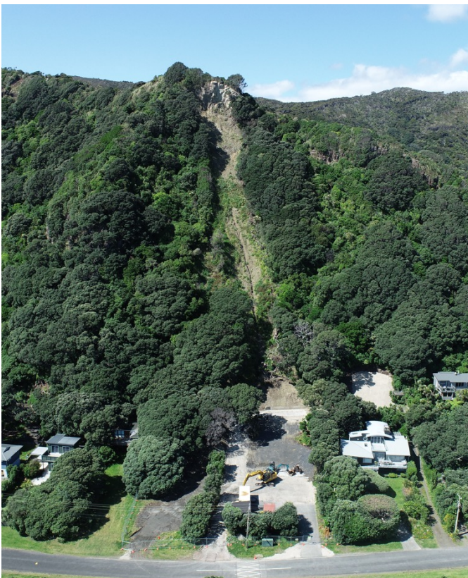
(FIGURE 43 AT LEFT) Translational slide that transitioned to rock avalanche and debris flow, head scarp and flow path (post-demolition). Head scarp at ridge crest exposes a faulted contact between Piha Formation and Waitarua Formation.
