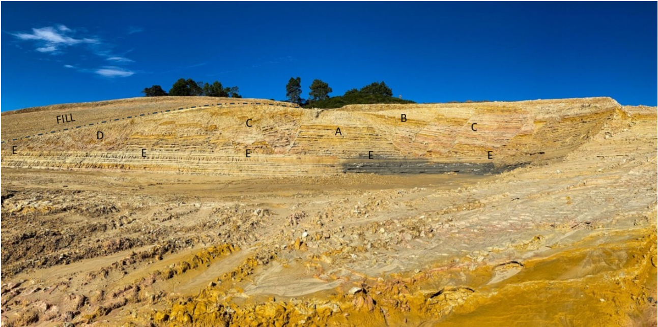
FIGURE 14: Slice through a translational relict landslide in East Coast Bays Formation Residual Soils, Orewa. Note landslide morphology features (A&B horst and graben structures, C- displaced blocks, D- increased downslope deformation and E- a basal shear surface separating lower undisturbed soil and overlying deformed, displaced soil.) The depth from ground level to the failure plane was observed to be 6 m.
