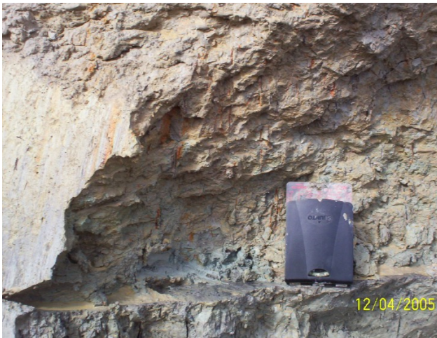
FIGURE 15: Pre-sheared surface and soil fabric in Northland Allochthon
