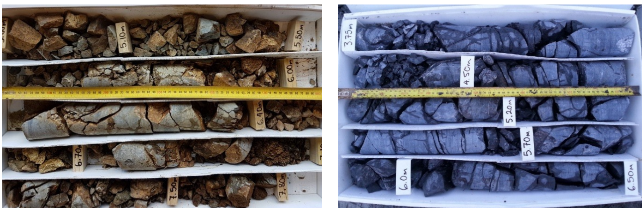
FIGURE 2: Typical closely fractured, weathered (left) and unweathered (right) rock core in Waipapa Group greywacke, Hunua Quarry
