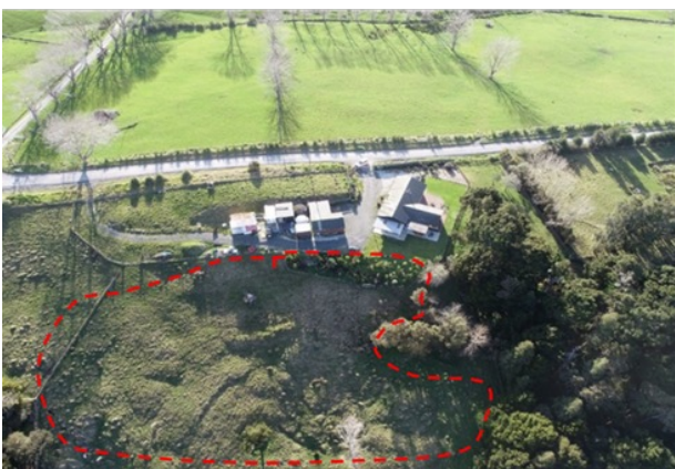
FIGURE 3: Examples of natural landsliding in Northland Allochthon terrain.
