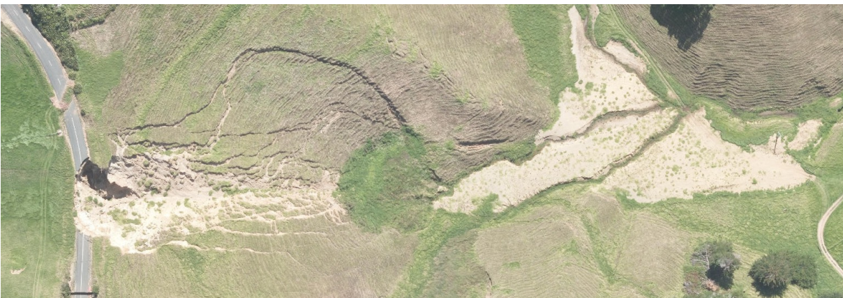
FIGURE 21: Debris flow in Kariotahi Group sand dunes (aerial view of Figure 7).
