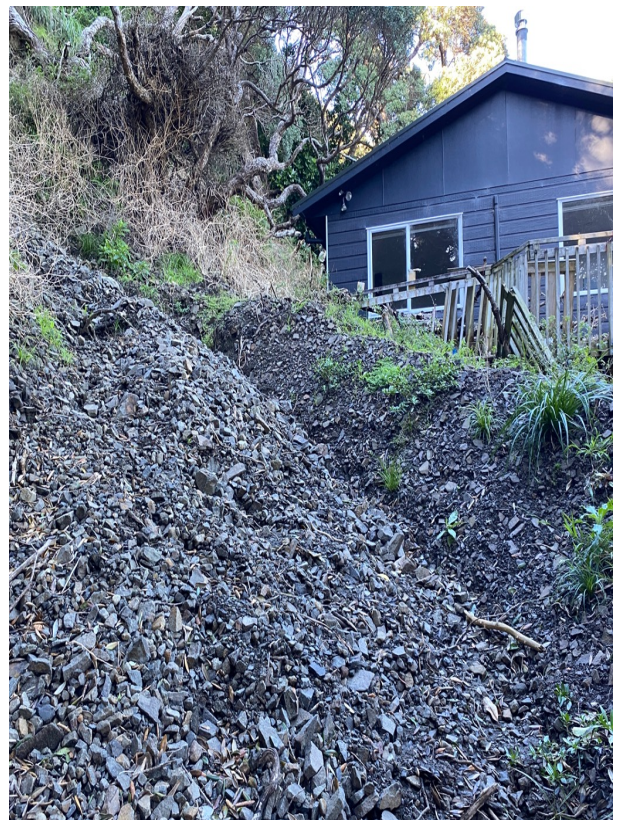
(FIGURE 43 AT LEFT) Translational slide that transitioned to rock avalanche and debris flow, head scarp and flow path (post-demolition). Head scarp at ridge crest exposes a faulted contact between Piha Formation and Waitarua Formation.
