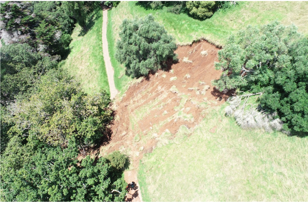
FIGURE 24: Debris avalanche in Auckland Volcanic Field sandy tuff soil.
