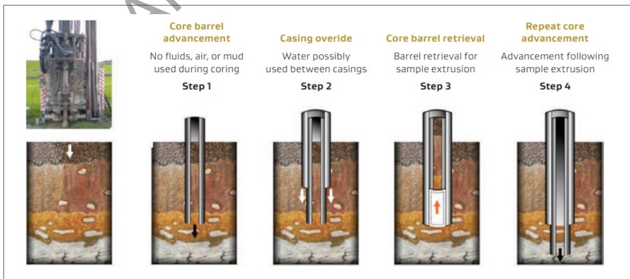
FIGURE 18: Typical sonic drilling sequence (NZGS & MBIE, 2021).
