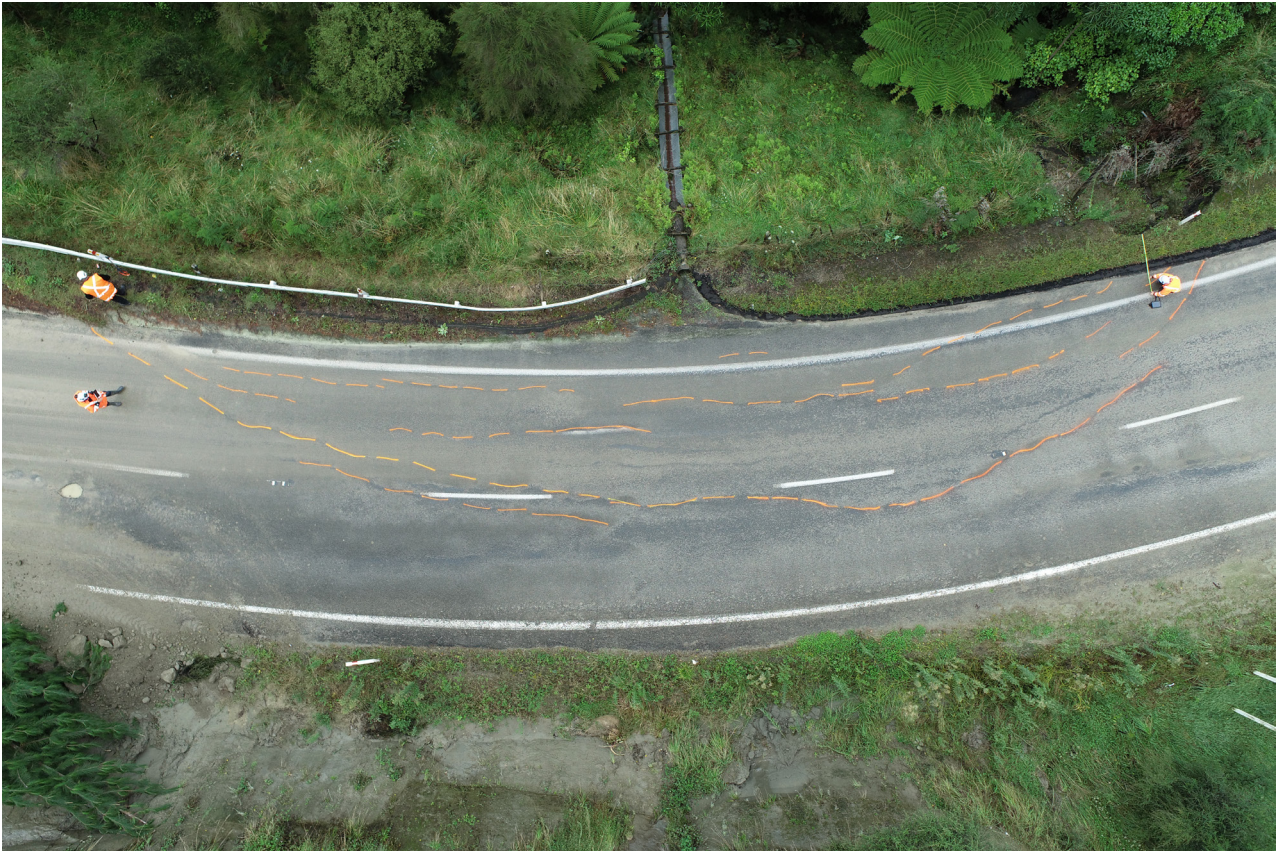
FIGURE 7. Marked up patterns of surface cracking and subsidence. Mapping the pattern of surface cracking and subsidence has clearly delineated the possible extent and head of potential future slope movement. Note: the road was closed at the time of the inspection.
