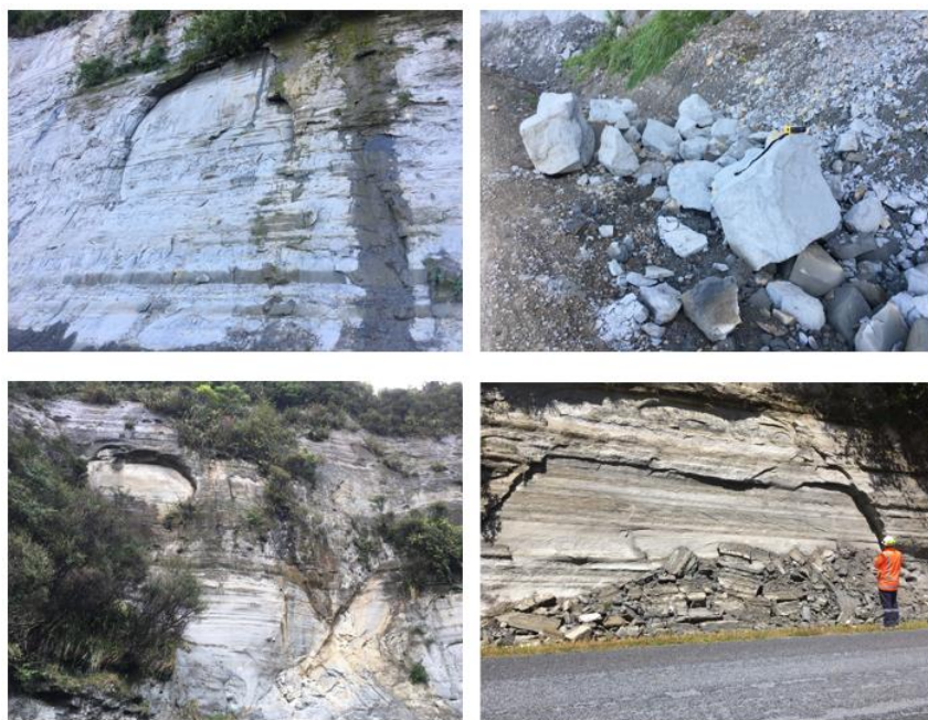
Figure 5: Slabbing failure examples from ‘papa’ rocks close to Mt Messenger.
