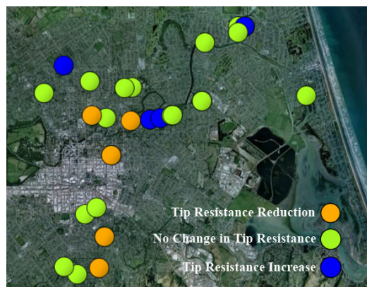
Figure 6: Mapped CPT tip resistance change for sites of re-liquefaction in Christchurch (50m maximum CPT offset)
