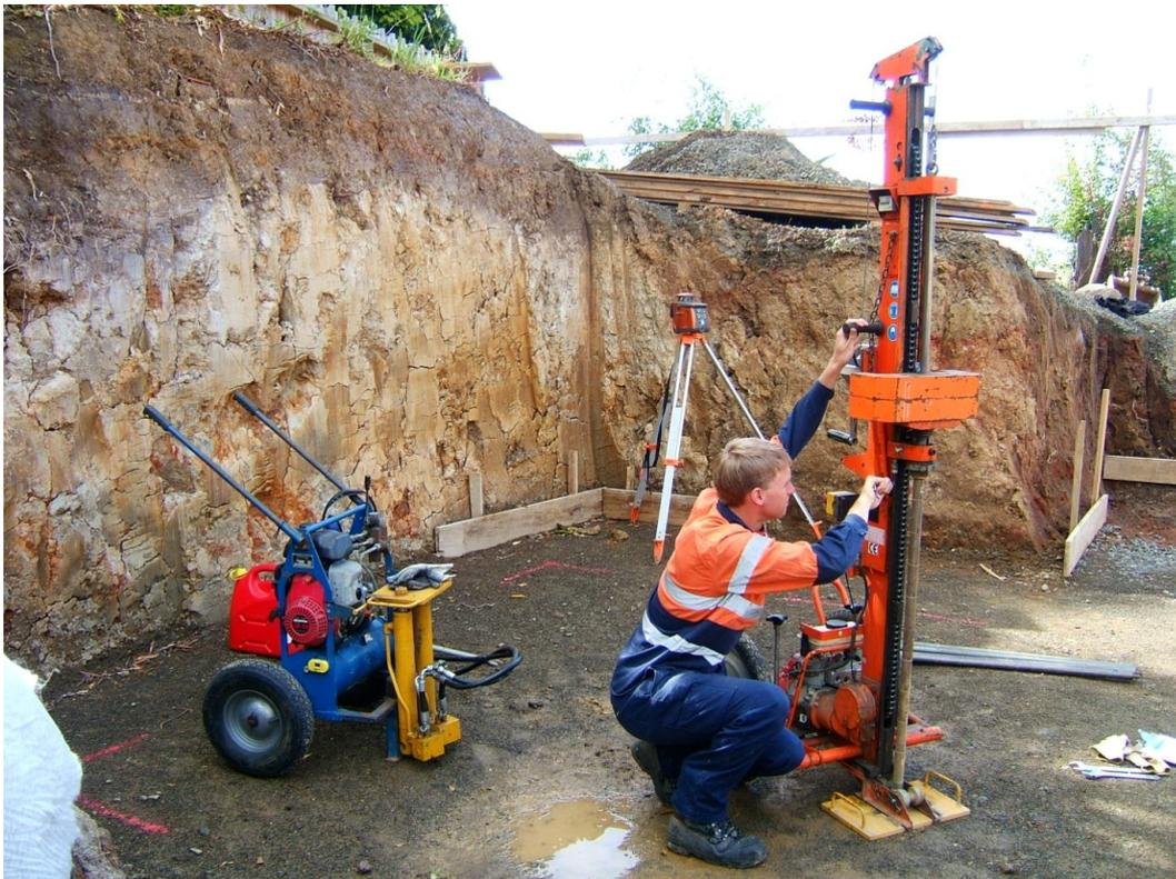
Figure 3: Dynamic Penetrometer
