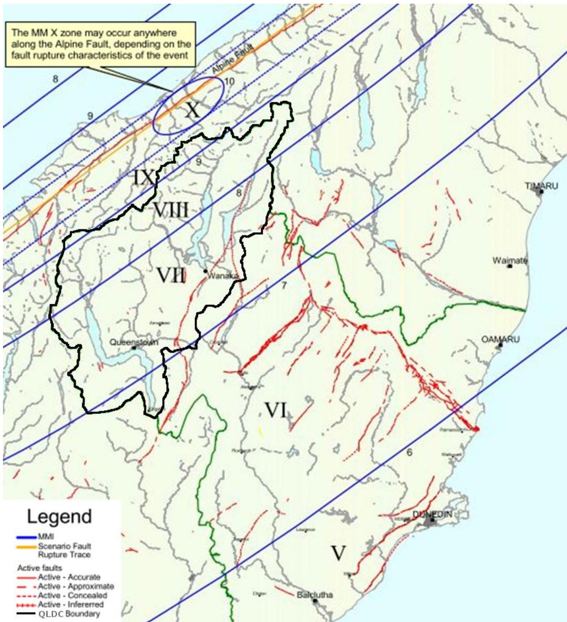
Figure 1: Isoseismals, Magnitude Mw 8.0 on the Alpine Fault (from ORC report, 2004)
