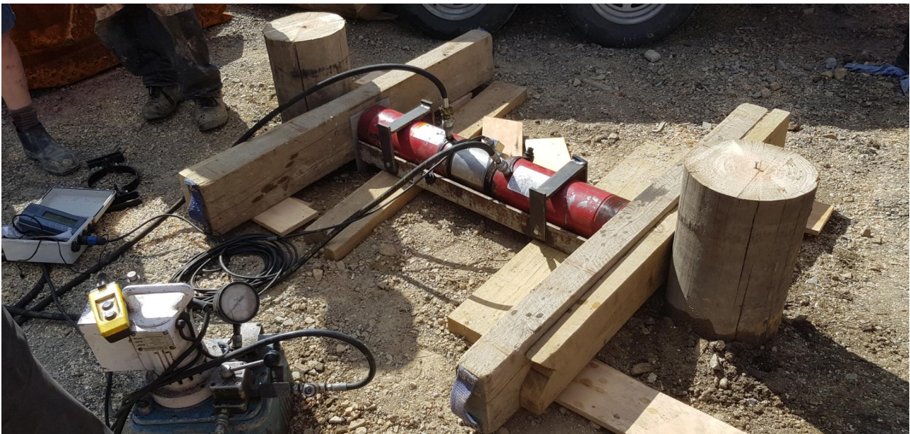
Figure 1: Lateral pile testing
