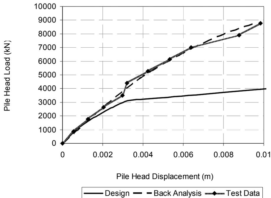
Figure 2: Bored Pile Test Data and t-z Analysis Results
