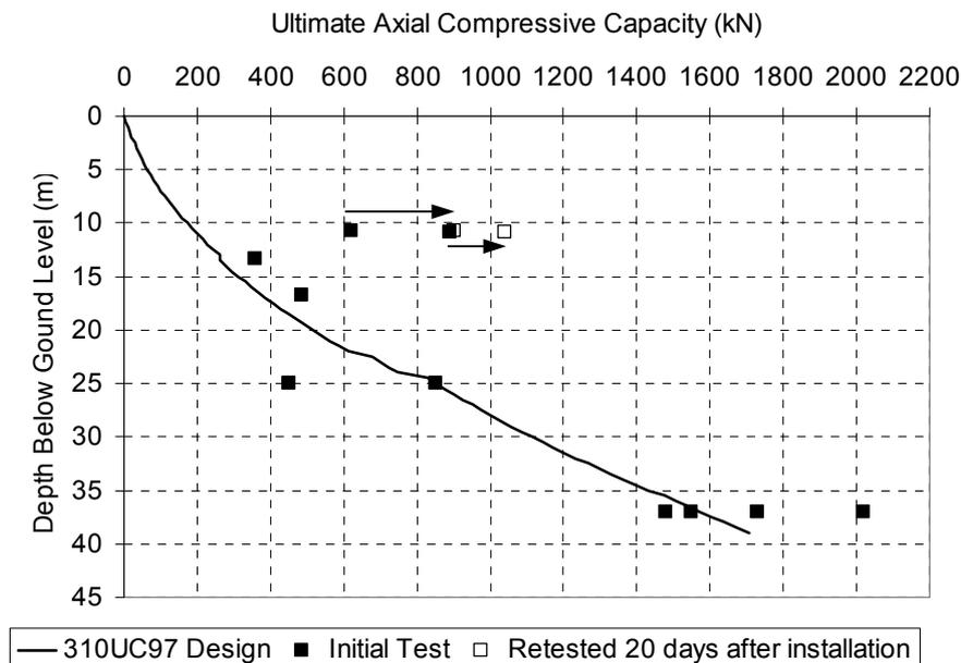
**Figure 1: H-Pile Test Results**
