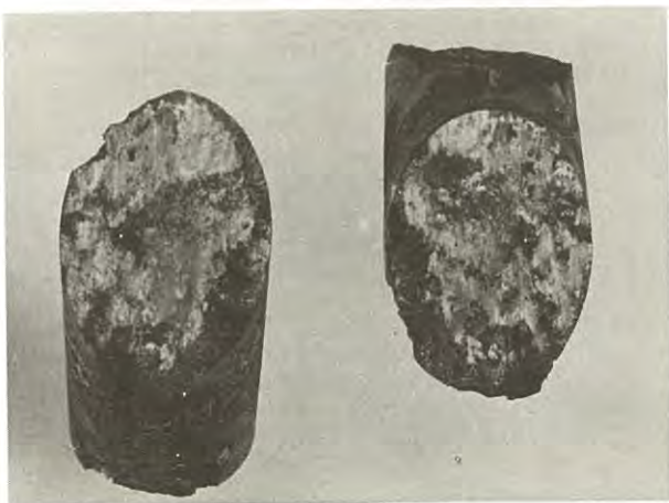
Fig. 6 A tested specimen showing joint surfaces.
