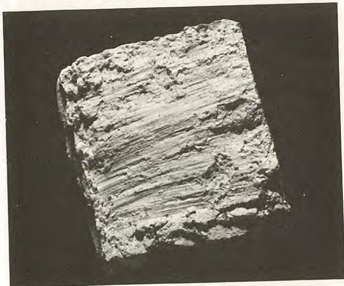
FIG. 10 Slickenside Formed in Remoulded Sample
