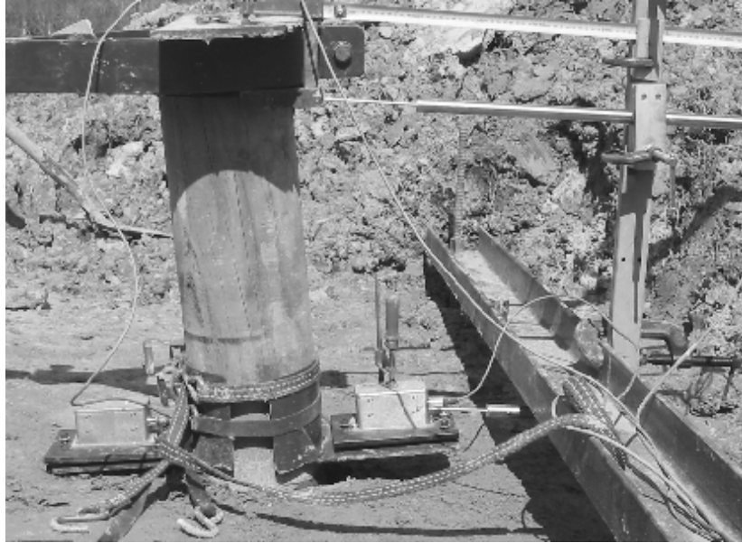
Figure 2: Pole under lateral load showing the instrumentation attached.
