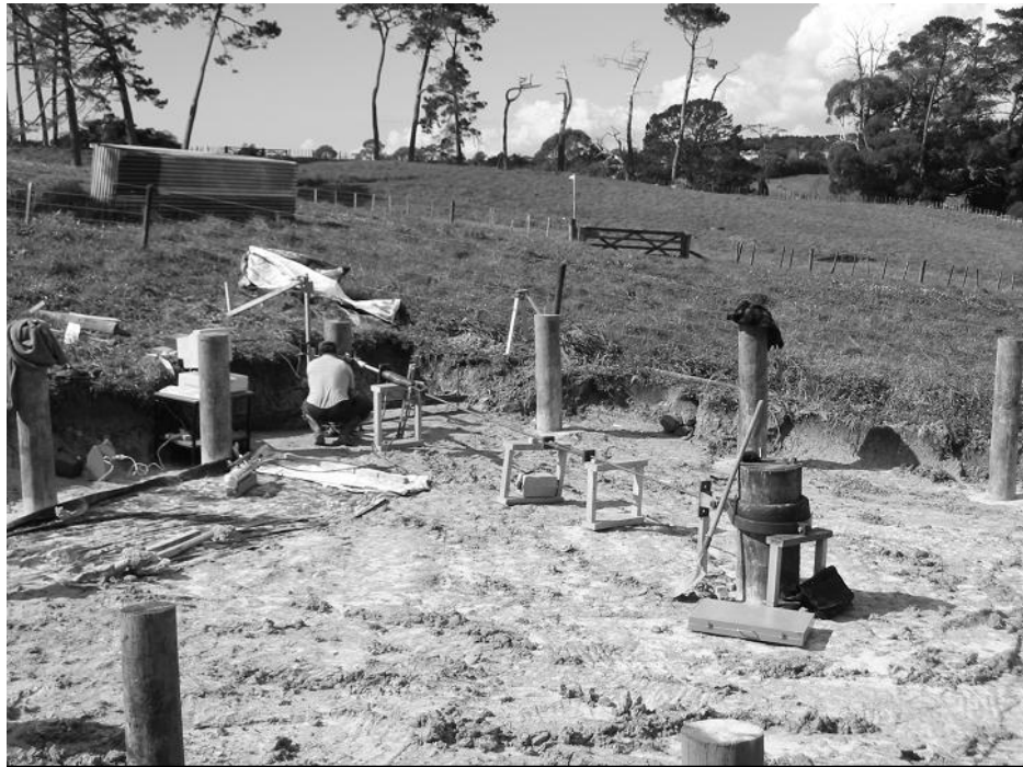
Figure 1: Layout of the site and test arrangement showing the centre reaction pole and the test poles around the periphery.
